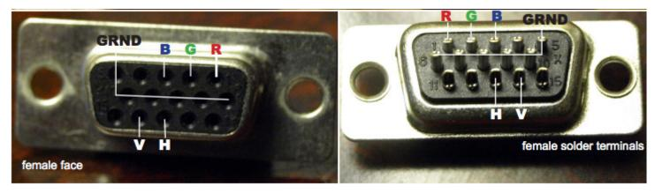
Note that the diagram above corresponds to the reverse side of the female d-sub connector (the solder terminal side). Be sure to double-check the numbered holes/terminals before soldering.
