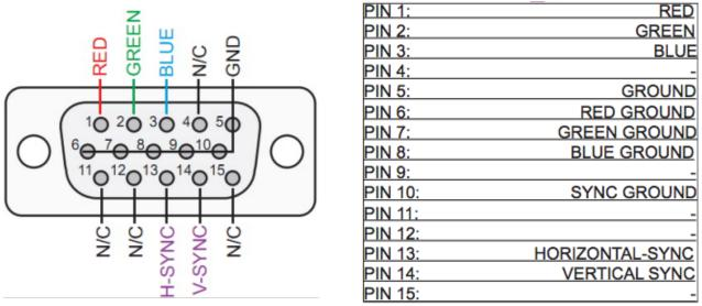
The VGA pin-out graphic above and its corresponding table show the function of each of the cable's 15 pins. This hack requires connecting the red, green, and blue video pins (pins 1-3) that drive their corresponding ray guns inside of the monitor, the ground signal (pins 5-8 and 10), the horizontal sync (pin 13), and the vertical sync (pin 14).
