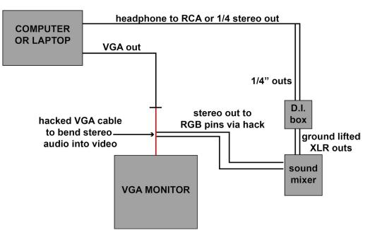
The above schematic is the basic RGB.VGA.VOLT system: a computer with a VGA output that connects to one single VGA computer monitor *after* the DIY VGA cable hacked to bend video into audio; the same computer is connected to a DI box via a 1/8" stereo to double 1/4" mono cable that then connects to a sound mixer; the sound mixer outputs its signal to the 1/4" jacks of the VGA cable hacked to bend audio into video.
