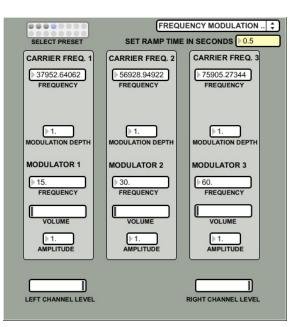
The third mode of sine wave synthesis is Frequency Modulation: modulating the frequency of a *carrier* frequency with a *modulating* frequency that is altered by a *modulation depth*. Frequency modulation produces tones equal to the carrier frequency plus and minus the modulating frequency.
