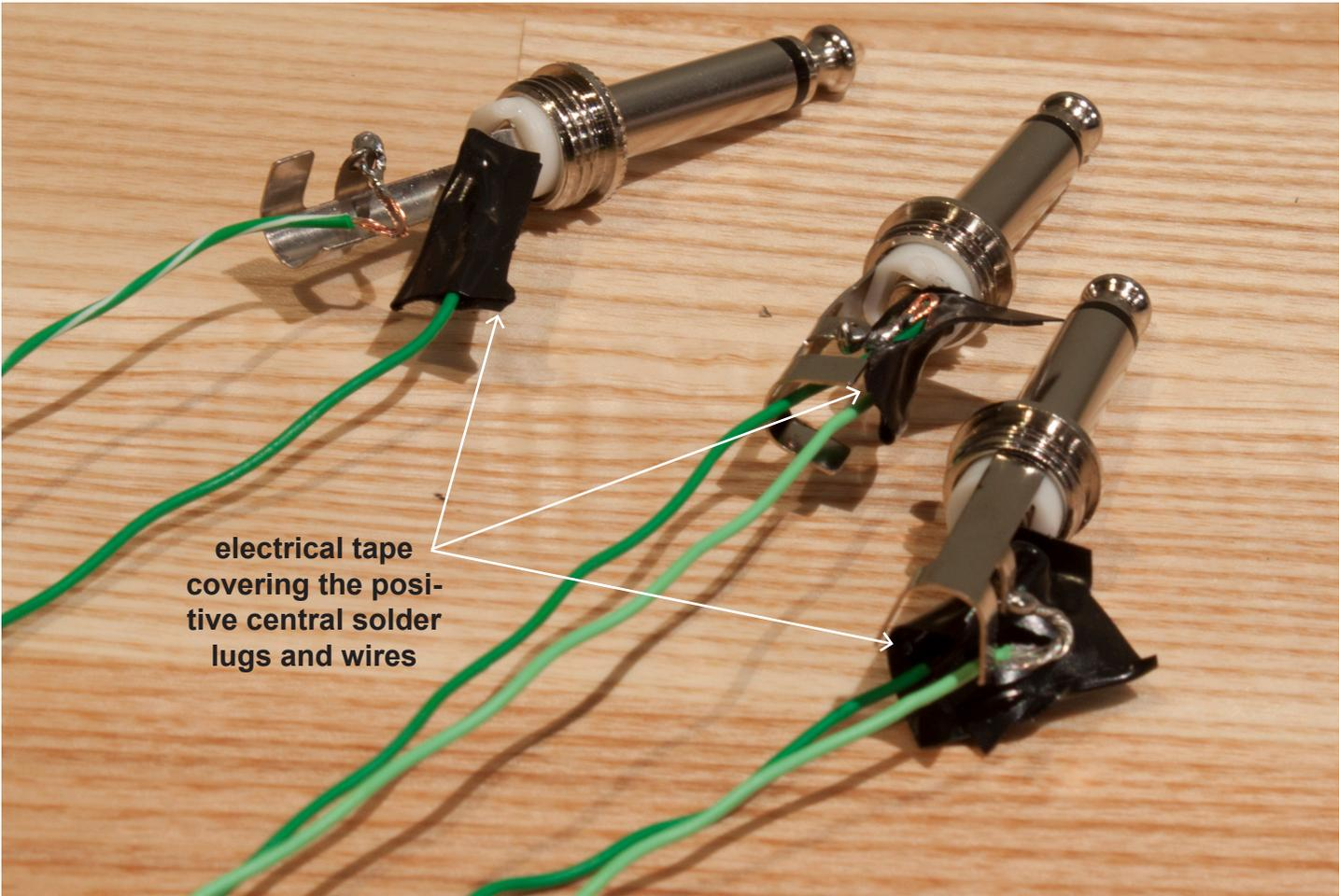
electrical tape covering the positive central solder lugs and wires
