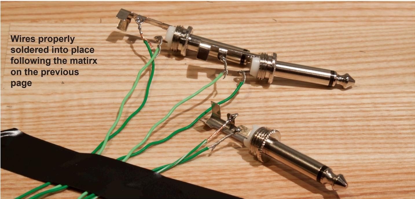
Wires properly soldered into place following the matrix on the previous page
