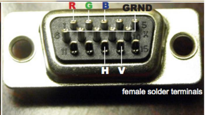
Note that the diagram above corresponds to the reverse side of the female d-sub connector (the solder terminal side). Be sure to double-check the numbered holes/terminals before soldering.
